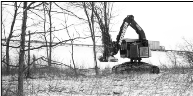
I want my own feller/buncher so I can restore habitat. This machine cuts off multiple trees at a time. Unfortunately, it's an expensive way to restore habitat. Photograph used with permission courtesy of the USFWS.
